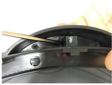
Step 2-2: The snap-fastenters can be seen when turning the lid over.
