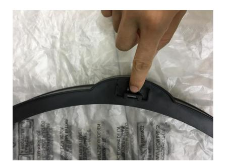
Step 3: Turn the lid back up, find a new latch, put it deep into the hole with a finger until a "clip" sound is heard.
